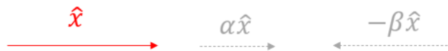
Fig. A1.1 The same vector escalated (in magnitude or in direction -negatively-).
