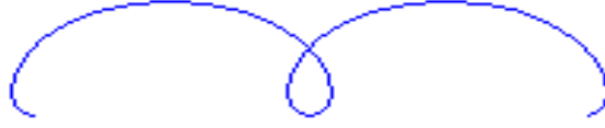
Fig. 6. The trajectory of an elongated cycloid. Because two cycles are depicted, the distance between the initial and final points of the trajectory is 2\lambda .
