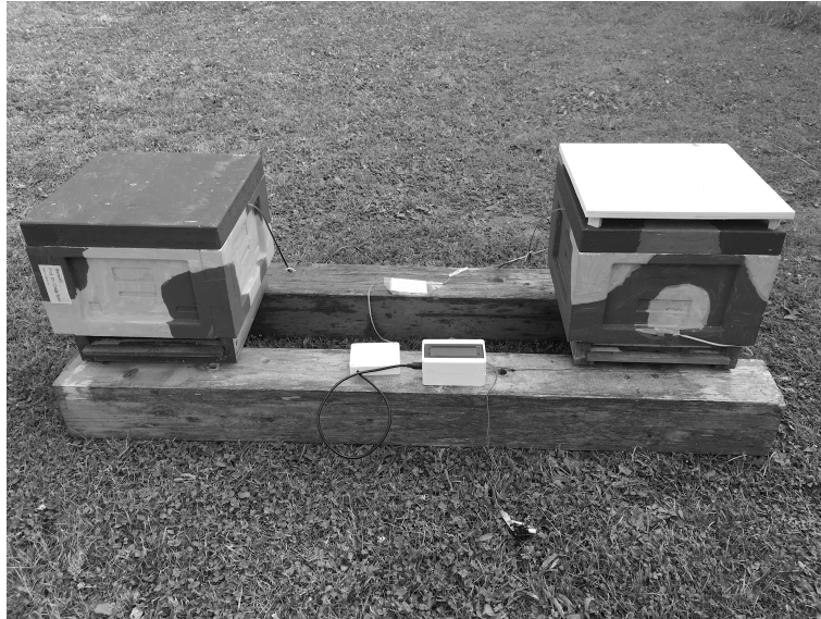
Fig. 6: Setup for the control measurement in hives without bees. Styrofoam hives in Mini Plus format are used. On the left side of the image is the hive without a radiation shield, and on the right is the hive with a radiation shield, which is ventilated by resting on square wooden blocks. The box in the middle contains the microcontroller for displaying temperatures. Temperatures are measured according to arrangement (a) in Fig. 3.
