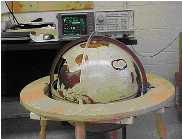
FIG. 2. (Color online) Photograph of the geomagnetic field sensor measurement setup.
