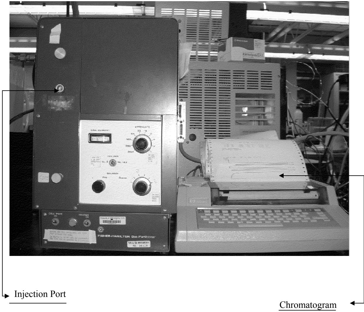
Figure 3.6. Fisher-Hamilton Gas Partitioner was used to measure ethylene.
