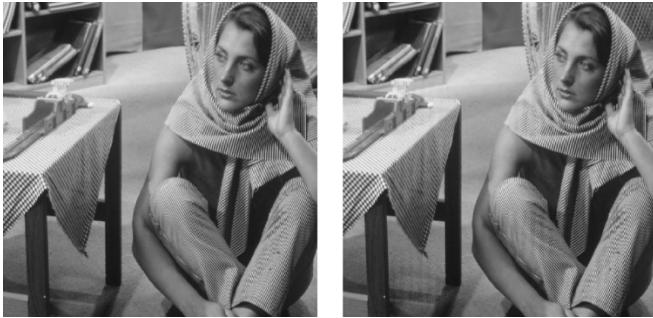
Fig. 7. Illustration of sample test images. Original Barbara (left) and Barbara watermarked using the proposed SLIDE watermark (right). PSNR = 38 dB.
