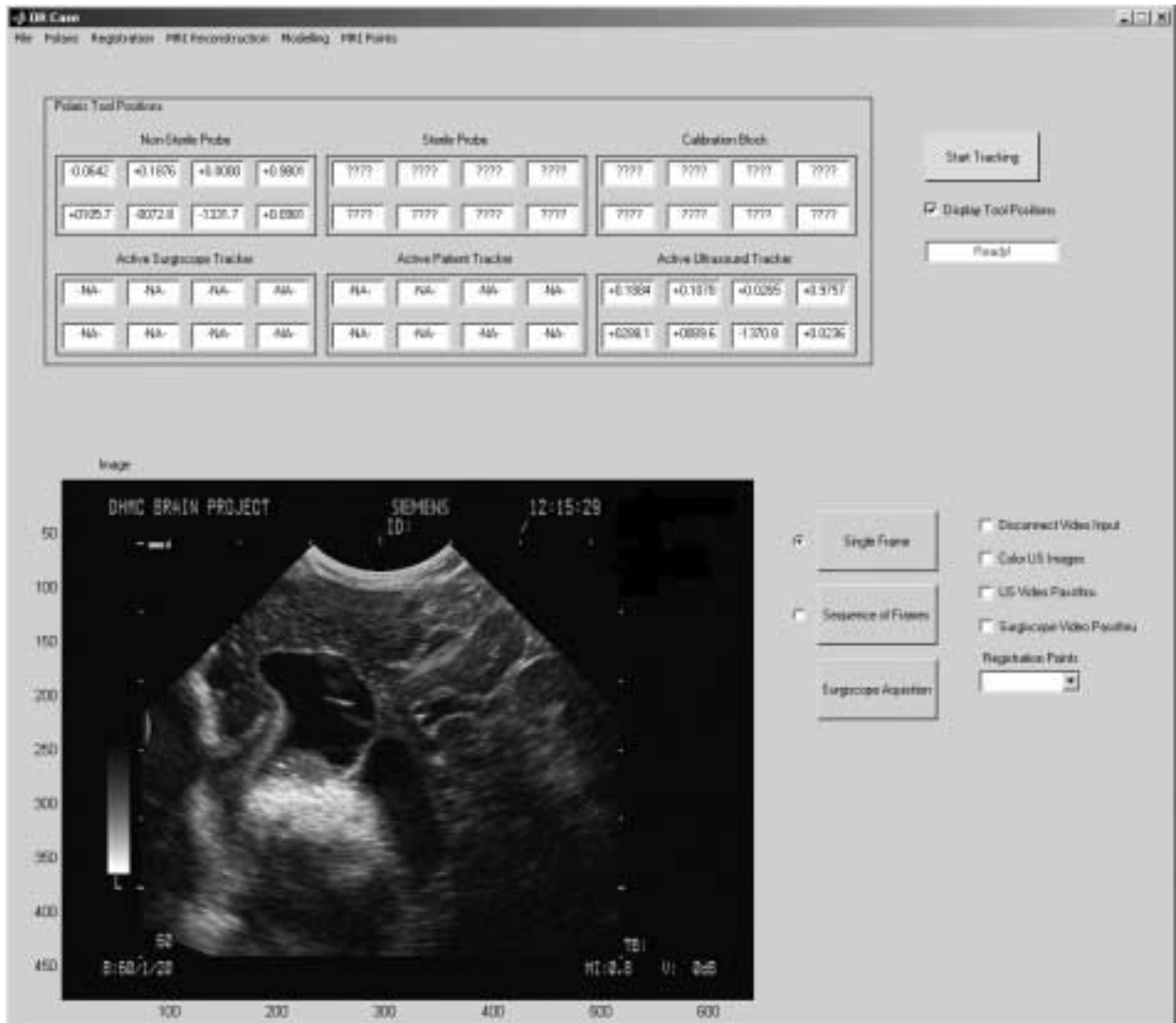
Figure 2: The main GUI window initiates communication with the 3D tracker, tracks tools and acquires ultrasound images. Other GUI windows can be called from the menu options at the top of the figure.
