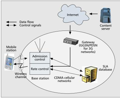
Figure 3. The architecture of the proposed framework.
