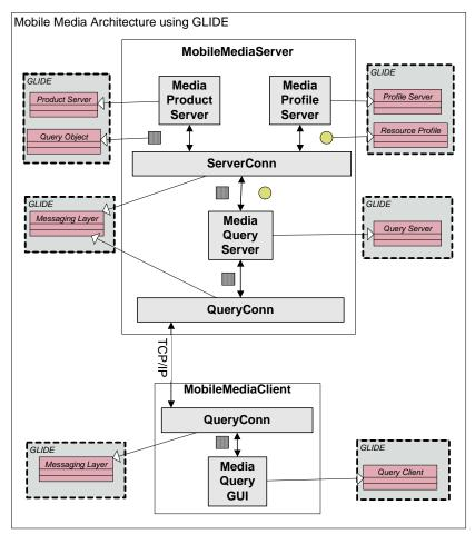
Figure 4. Mobile Media Application Architecture
