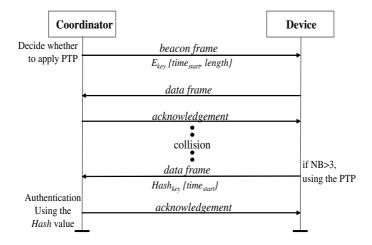
Fig. 6. Process for channel acquirement
