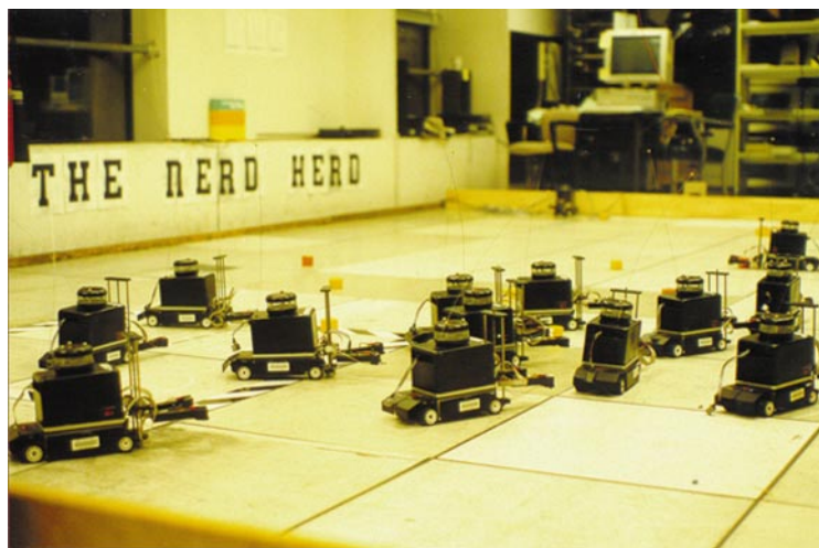
Fig. 1 The nerd herd. A group of 13 flocking mobile robots. These robots also demonstrated wandering, following, aggregation, dispersion, chain-formation and foraging.
