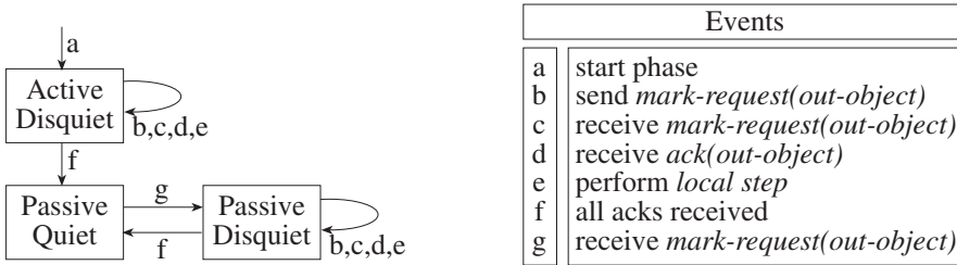
Fig. 5. state transitions for termination detection. An additional initial state required by pto’s that receive a scan-request before the instruction to start the scan phase is omitted for simplicity.
