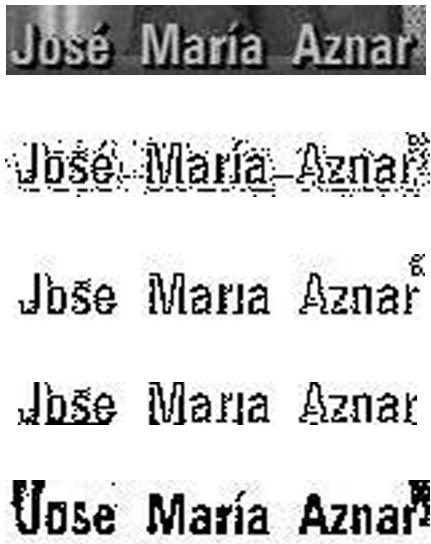
Fig. 2. (a) The original sub-image, (b) edge image, (c) accepted connected components, (d) CCs merged in the same text box, (e) locally thresholded image containing text as black on white.
