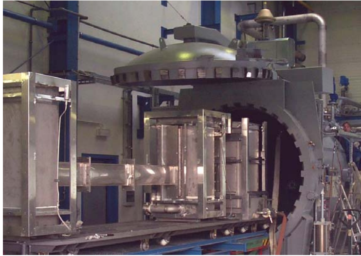
Fig. 36 TOPFLOW "Diving Chamber", view from the side of the full-size port, hot-leg test without thermal insulation and still without steam generator inlet chamber
