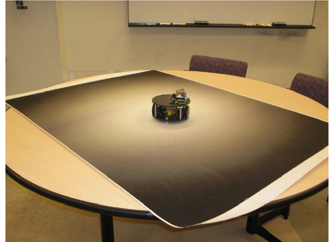
Fig. 7. The mobile robot in Fig. 6 will be made to seek the extremum on a printed paper surface, which varies in color from white in the center to gray to black away from the center.
