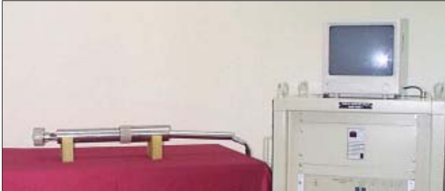
Gamma scanner for fuel pin (above) and Miniature underwater radiation resistant closed circuit television (CCTV) Camera developed at BARC, for remotised inspection of coolant channels of PHWRs
