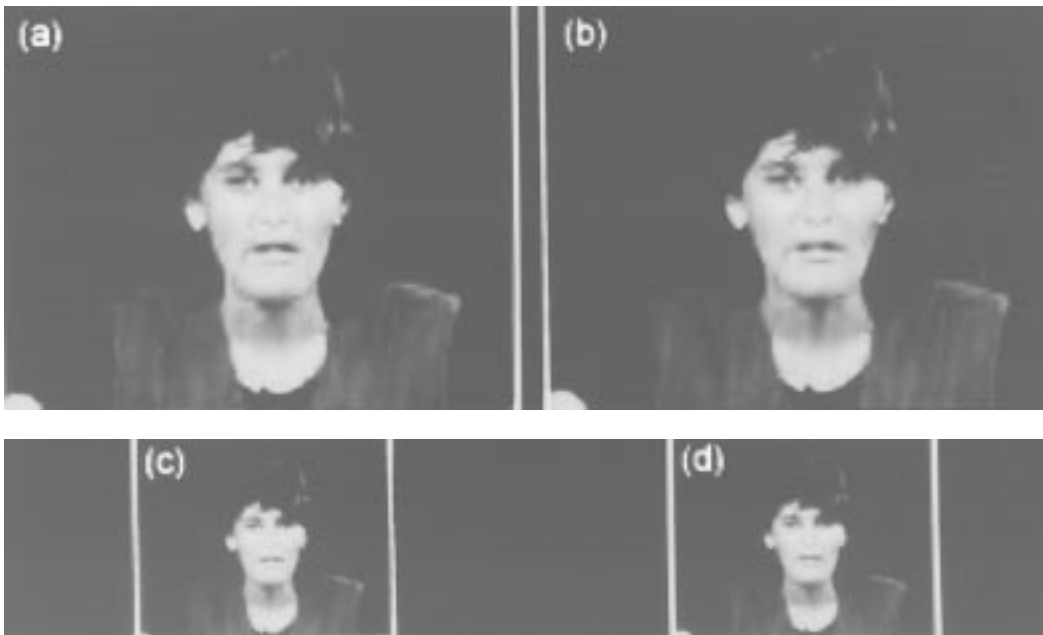
Fig. 19. Multiresolution video scalability: Miss America frame 32 using TRI-ZTR at 10 Kbits/s. (a) Full spatial and full temporal resolution, (b) full spatial but half temporal resolution, (c) half spatial but full temporal resolution, and (d) half spatial and half temporal resolution.
