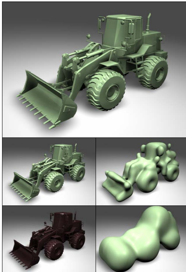
Figure 1: Interpolating and approximating surfaces (green) generated from polygonal original (brown).
