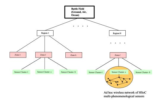
Fig. 5 Multi-level networking of the HSoCs
