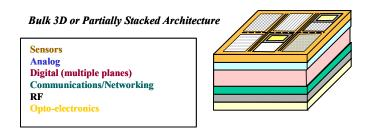
Fig. 2 3D Heterogeneous System on a Chip
