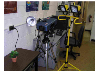
Figure 8. Experimental setup using SOC 700 hyperspectral camera
