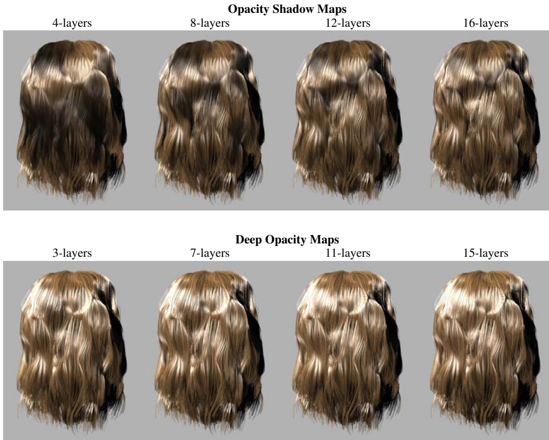
Figure 2: Dark hair model for qualitative comparison. Layering artifacts of Opacity Shadow Maps generate dark diagonal stripes, while Deep Opacity Maps generate similar images with any number of layers.
