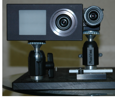
Figure 5. Our data capture setup, consisting of a depth camera and a color camera.
