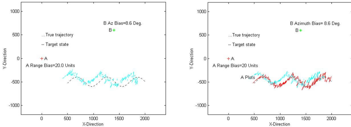
**Figure 6.** Tracking with range and azimuth bias registration using GLSE for bias estimation.
