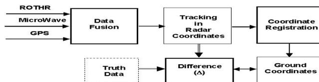
**Figure 1.** Integrated Data Fusion Flow for Relocatable Over-the-Horizon Radar (ROTHR).
