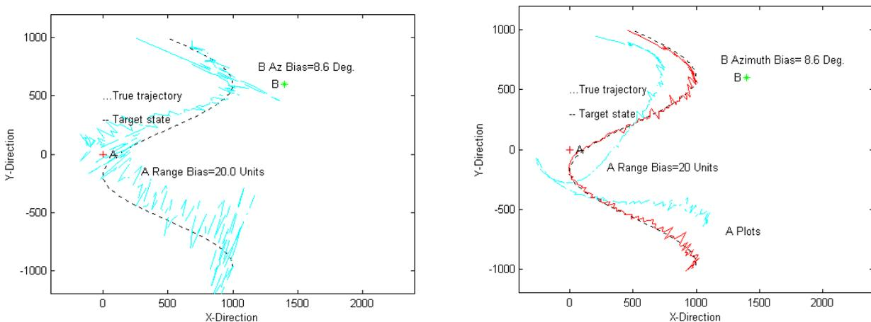
**Figure 7.** Tracking with range and azimuth bias registration using GLSE for bias estimation.
