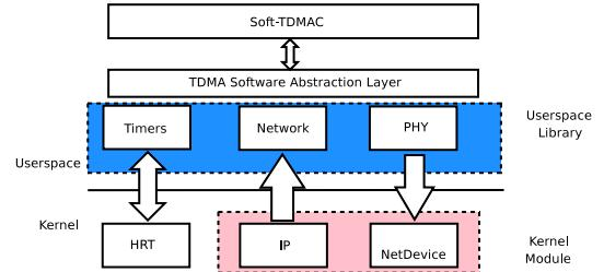
Fig. 3. Soft-TDMAC Architecture
