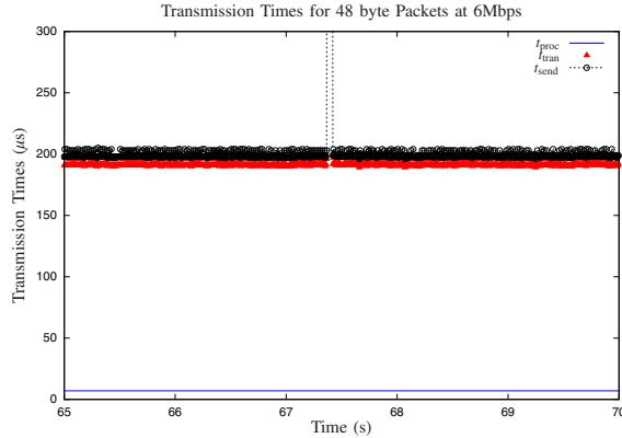
Fig. 4. Transmission Delay
