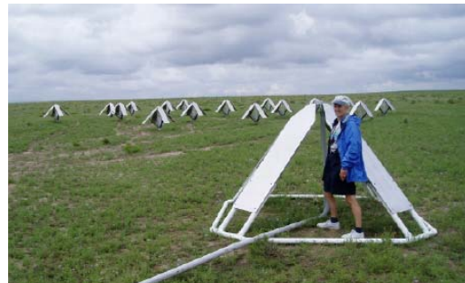
Figure 4. A prototype Long Wavelength Array antenna. This antenna is sensitive to the frequencies relevant for probing the Dark Ages. The final antenna design has manufacturability as a criterion in its design, and will be somewhat lower in mass, but remain too massive for a lunar mission. In the background are the antennas of the Long Wavelength Demonstrator Array.
