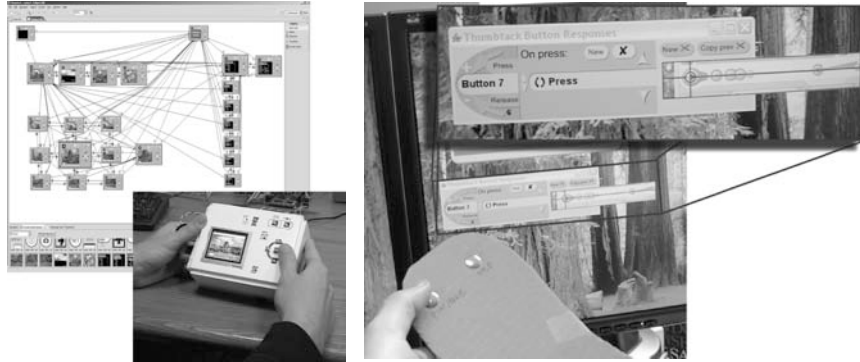
Figure 12. Two design tools: Left: The d.tools software editor and an interactive prototype built in approximately 3 hr (Hartmann et al., 2006). Right: With BOXES, designers can prototype physical forms in minutes and then rapidly add simple functionality to them by connecting thumbtacks to on-screen mouse and keyboard actions (Hudson & Mankoff, 2006).
