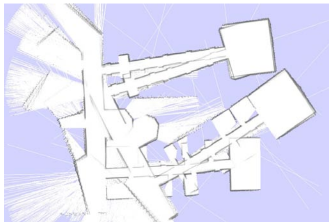
Fig. 10. Map obtained using odometry and laser data without correction.
