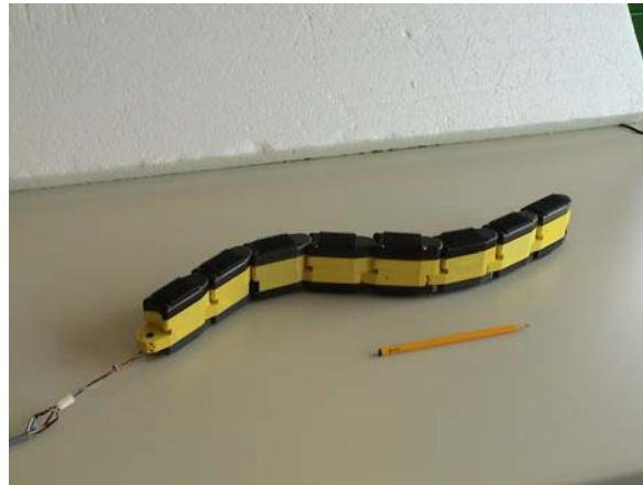
Figure 4: AmphiBot I (Courtesy of Alessandro Crespi, Biologically Inspired Robotics Group at Ecole Polytechnique Fédérale de Lausanne)
