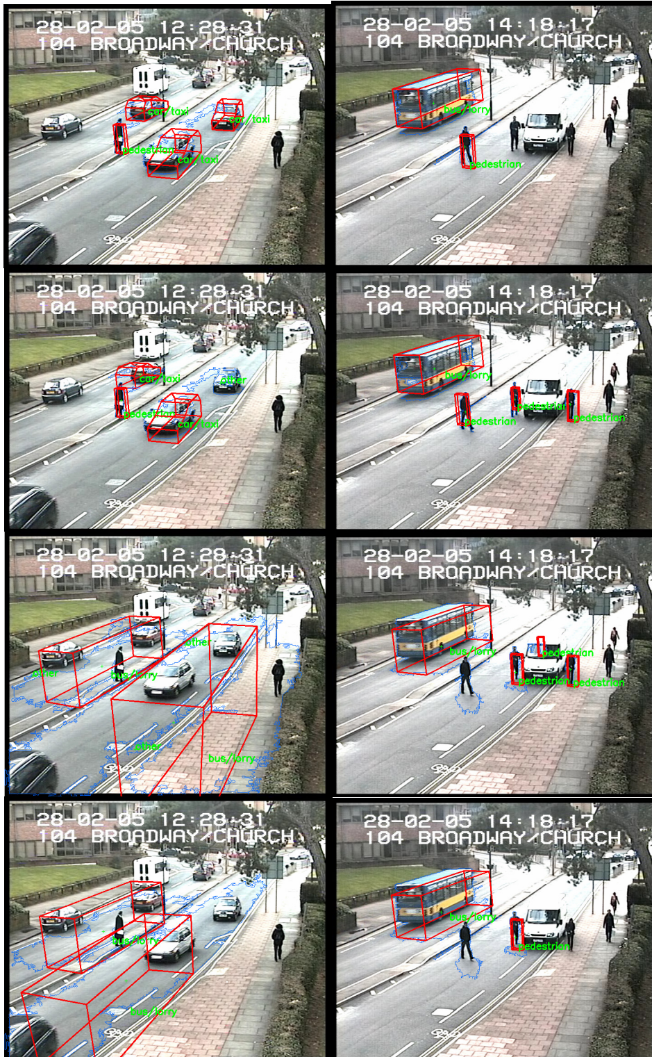
Figure 9 Two example views of the combined vehicle and pedestrian framework for 4 different filter configurations from top to bottom: shadow removal (Sr), shadow removal with de-interlacing (Sr+Di), de-interlacing (Di) and no filter (-). Too large silhouettes can be observed without shadow removal causing missed vehicles and wrong classifications (last two columns).
