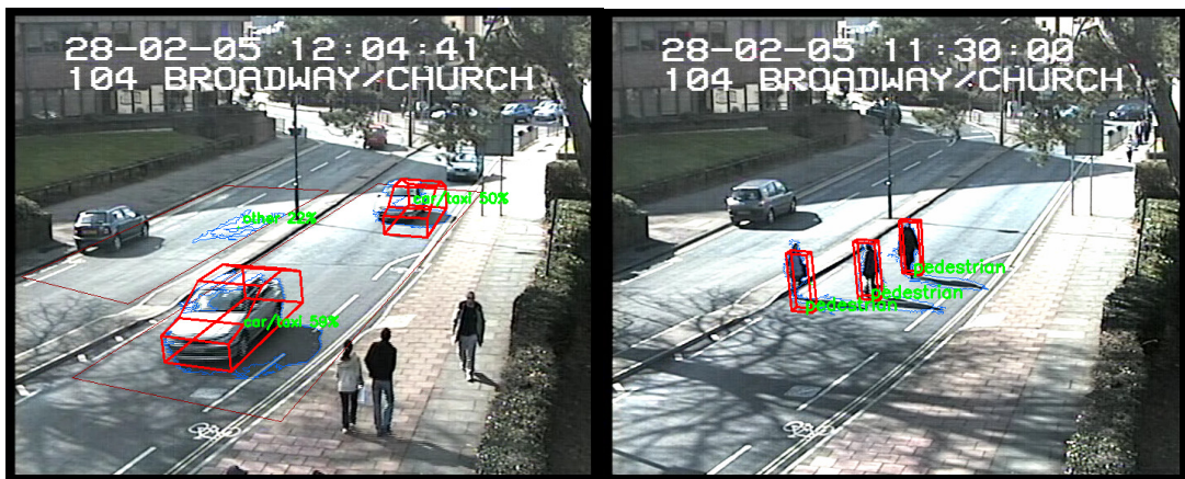
Figure 1 Example views from the i-LIDS data set with active windows and detected vehicles and pedestrians
