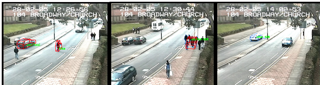
Figure 7 Two examples for false positives due to pedestrians being detected as bike and as car due to occlusion in a group. The last image shows a missed car due to its similar colour compared to saturated road area
