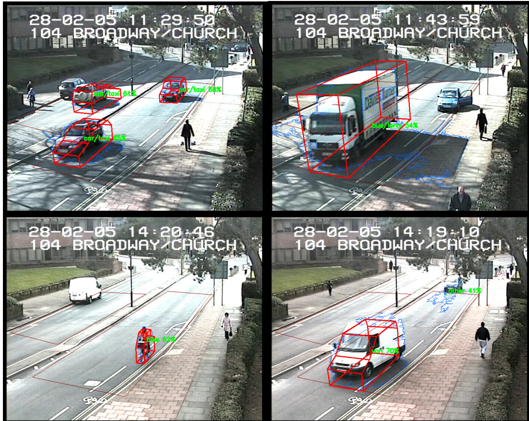
Figure 6 Examples of correct detections and classification of vehicles using the shadow removal filter
