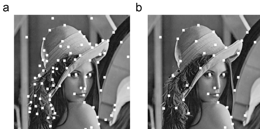
Fig. 1. The effect of different window sizes on the feature points. (a) Window size of 26 \times 26 and (b) window size of 52 \times 52 .
