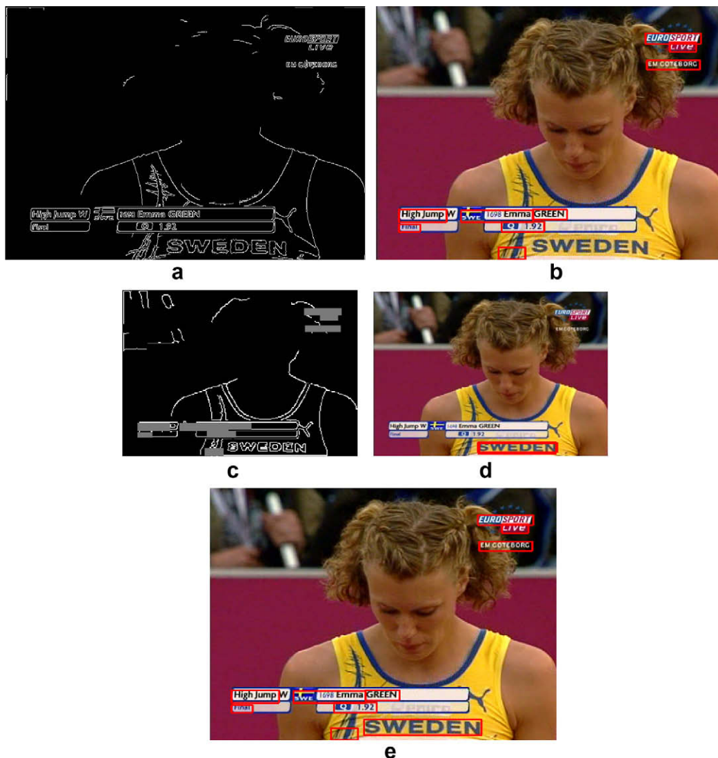
Fig. 16. Multiresolution analysis. (a) Original resolution edge map, (b) result at original resolution, (c) low resolution edge map (gray pixels denote the area of the already found text), (d) result at low resolution, (e) final result.
