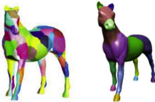
Figure 2. Patch-type (left) and part-type (right) segmentation taken from [15].
