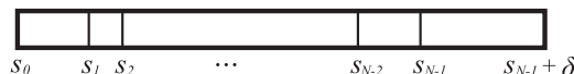
Fig. 9. Loopback cache: the chain buffers an extra s_{N-1} - s_0 + \delta seconds of data.
