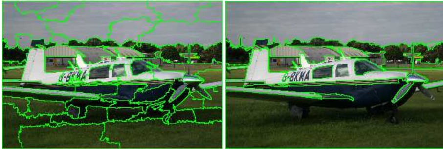
(c) Synergistic Segmentation [7] - 45.3 segments per image on average (d) Graphseg [10] - 21.1 segments per image on average
