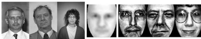
Fig. 2. Left: Original samples in the FERET database. Middle: The standard mask. Right: The samples after the preprocessing sequence.
