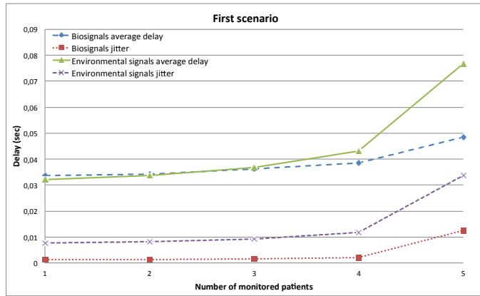
Figure 1. Signals delay and jitter vs. number of monitored patients for simple patient monitoring case.
