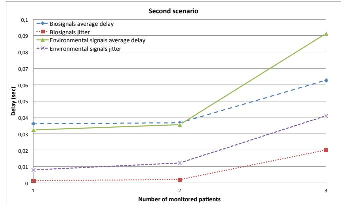
Figure 2. Signals delay and jitter vs. number of monitored patients for moderate patient monitoring case.
