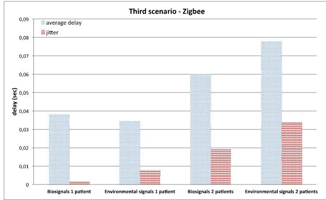
Figure 3. Signals delay and jitter vs. number of monitored patients for advanced high capabilities patient monitoring case – Zigbee serving as PAN.
