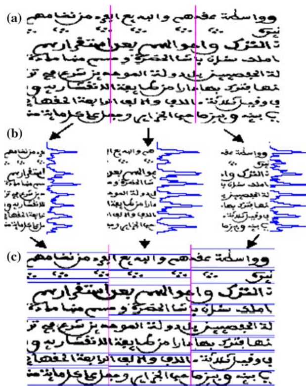
Fig. 1 Block extraction on a sample document: a dividing the document into strips. b projection profiles within each strip c resulting text blocks (a text block is delimited by two horizontal blue lines)
