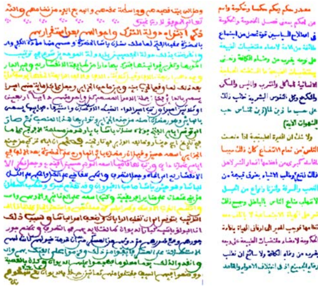
Fig. 19 Text-line segmentation of the TSD document in Fig. 12a and of the WSD document in Fig. 16b
