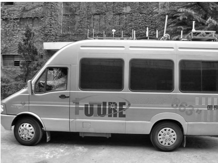
Figure 2.13 The test vehicle of the FuTURE TDD trial system.
