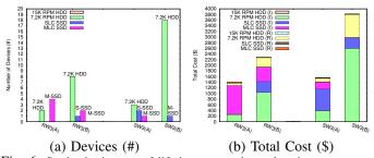
Fig. 6: Study the impact of lifetime constraints taken into account. "A" and "B" in the parenthesis denote "without lifetime constraint" and "with lifetime constraint" respectively.
