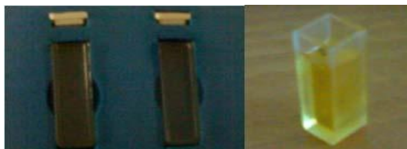
Fig.1. Cuvette holders with heptane and oil
