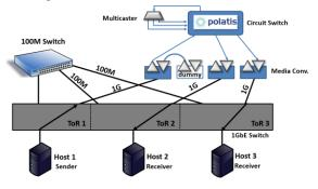
Fig. 2. End-to-end experimental testbed.
