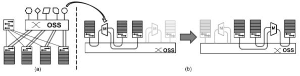
Fig. 1. (a) Hybrid network architecture featuring various photonic capabilities, as represented by the polygons. (b) Utilizing the optical space switch to dynamically deliver optical layer multicast between different racks in a data center.
