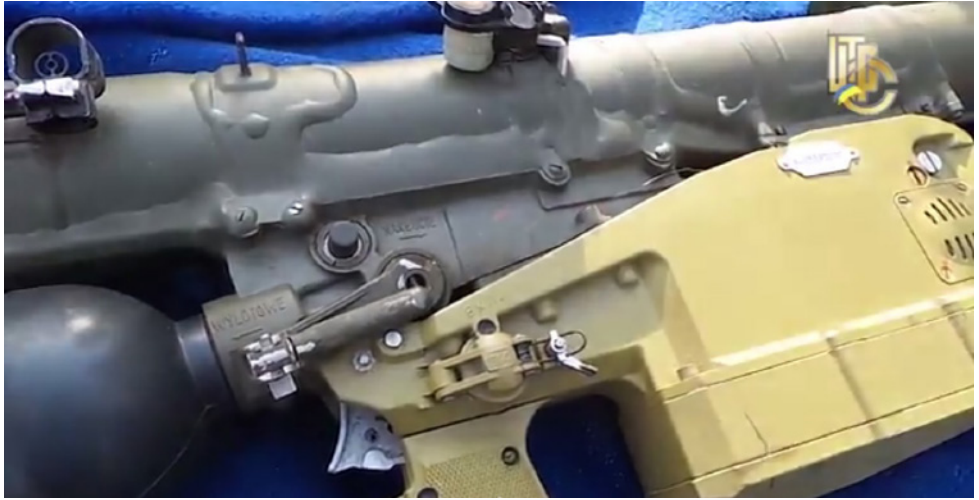
Photo 62 A Polish PPZR Grom E2 missile tube fitted with a Russian 9P516 gripstock. Photo credit: Ukraine Military TV
