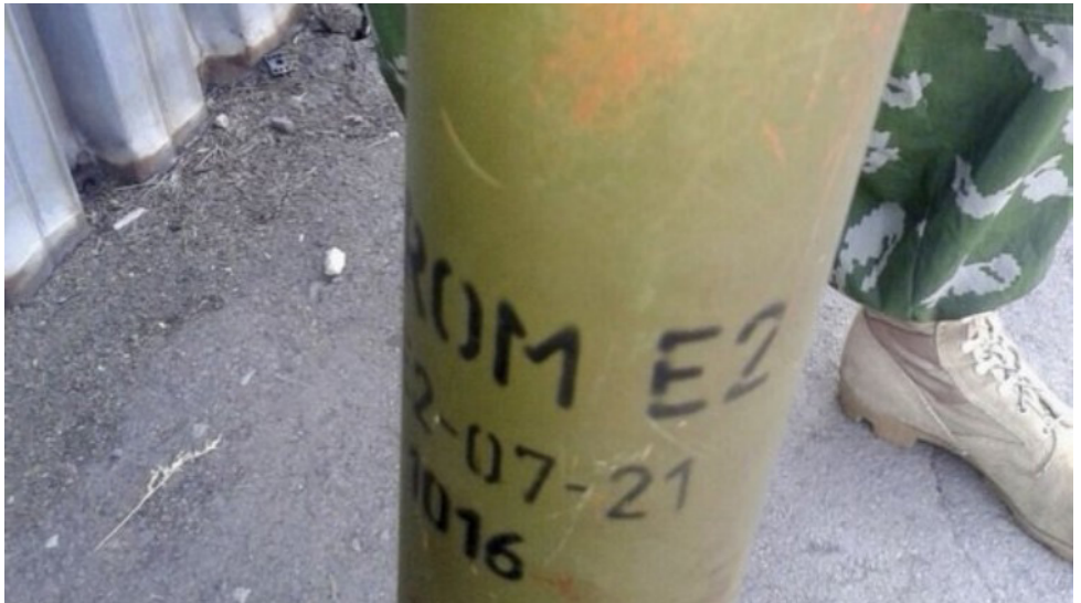
Photo 63 Close-up of markings on a Polish PPZR Grom missile tube, clearly showing the 'GROM E2' designation and indicating that the missile was produced in 2007. Photo credit: Ukraine Military TV
