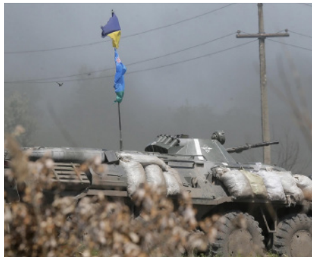
Photo 87 Ukrainian security forces operating a BTR-80 APC with sandbags acting as improvised armour.
