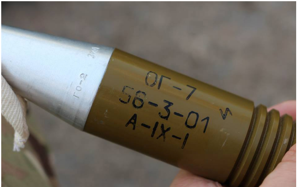
Photo 49 An OG-7 HE-FRAG projectile produced in Russia in 2001, fitted with a GO-2 fuze, produced in Russia in 1992. Photo credit: 'Pasha K.'
