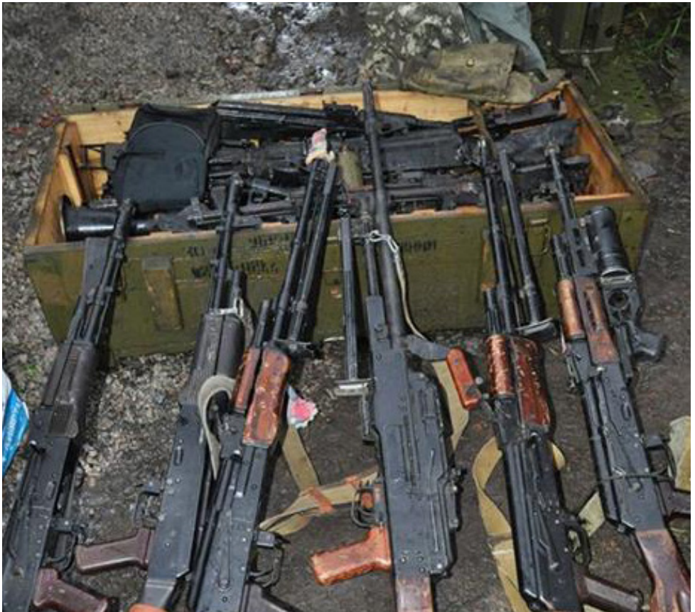
Photo 18 A representative range of Kalashnikov rifle and machine gun types in pro-Russian militia service. These examples were allegedly captured from fighters of the 'Donbass People's Militia', in June 2014. From left to right: late 1980s production AK-74 with 'plum' coloured polymer furniture (x 2), RPK-74, PKM, RPK-74 and 1970s-80s vintage AK-74 with wooden furniture and fitted with GP-25 underbarrel grenade launcher.
