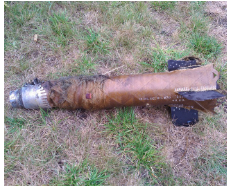
Photo 101 A 95Ya6 booster rocket used with the 57E6 series of SAMs, as well as other missiles.
