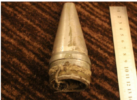
Photo 91 A TM-120 mechanical time fuze which failed to function. Eastern Ukraine, November 2014. Photo credit: Harriet Salem / VICE News
