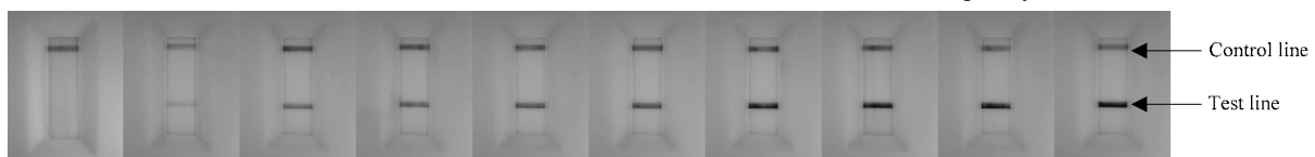
Figure 5. Images of gold immunochromatographic strip of different concentration (from the left side: 0, 10, 35, 75, 100, 150, 200, 300, 400, 500 mIU/ml)
