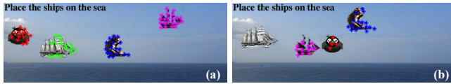
Fig. 5. KLT tracking. (a) Initial corner points on the moving objects; (b) KLT loses tracks on the “white ship” after 30s (10 fps).
