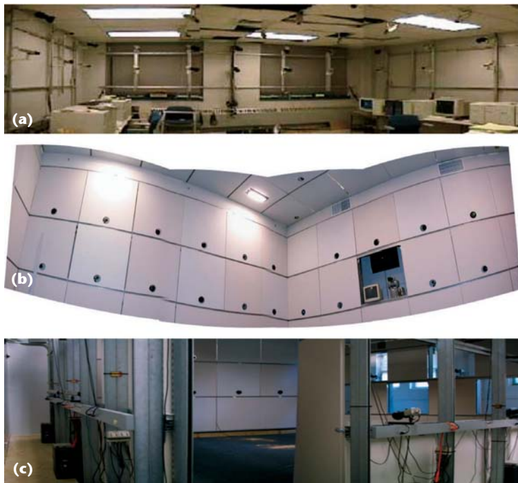
3 (a) The 3D Room setup with digital capture (circa 1998). (b) A panoramic view of the current Virtualizing Studio (circa 2002) with 48 cameras and full digital capture. (c) The outside view of the Virtualizing Studio.
