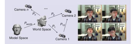
[FIG2] Model-based face tracking from one or multiple cameras.  $P_{world}$  is the transformation from model space to world space;  $P_n$  is the projection of the face model to the *n*th camera;  $P_{ij}$  is the transformation between cameras. All these parameters are estimated automatically in the algorithm.
