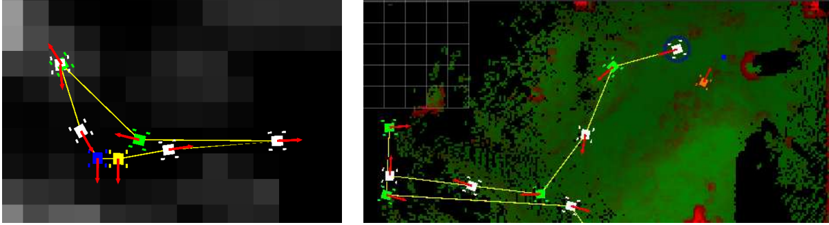
Figure 8: Left: Pre-mission planning on a rough height map. Right: Interactive plan refinement on an updated height map. Red cells indicate that the height of the refined map deviates by a great amount from the rough heightmap. This information is used by the operator to align the two maps precisely.
