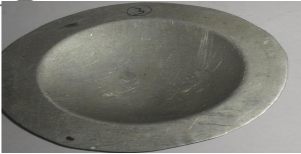
Fig. 4: Deformed piece through the SHF setup.
