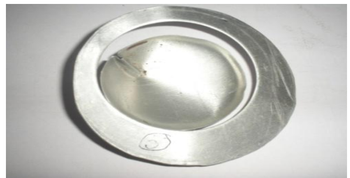
Fig. 8: Wrinkling and tearing of Aluminium work piece
