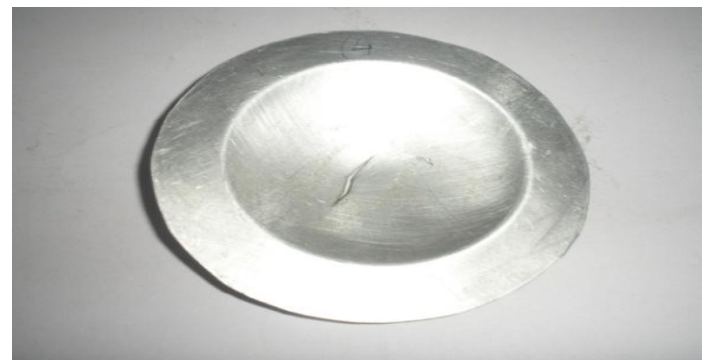
Fig. 9: Wrinkling and Bursting of Aluminium work piece.
