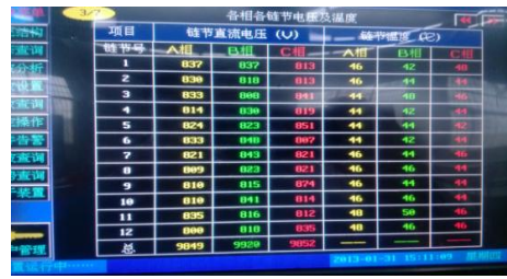
Figure 16. Experiment results of capacitors voltage
