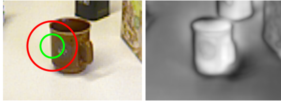
Fig. 2. Common-border Saliency: The Difference-of-Gaussian (DoG) operator that is used to compute center-surround contrasts has a low response when located at object boundaries (green = center, red = surround of the DoG filter).
